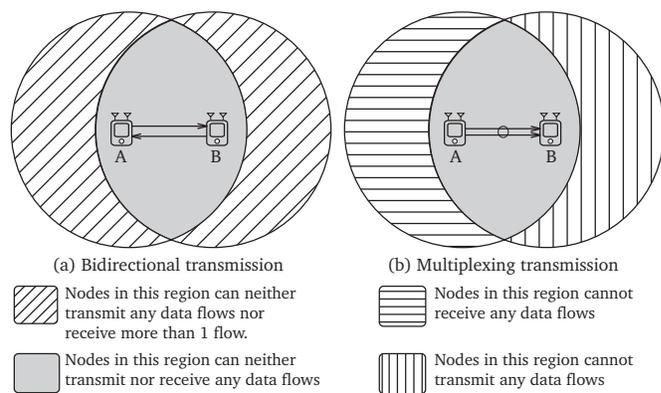
Fig. 2. The interference footprint of the transmission between node A and node B in a wireless network where each node has two active RF chains and can enable either full-duplex or MIMO transmission. The circle around node A/B indicates its interference range. In (a), both node A and node B are operating in full-duplex, and a bidirectional transmission is established between the two nodes; in (b), two spatially multiplexed streams are sent from node A to node B.
