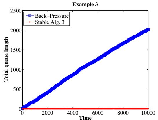
(b) Comparison of MaxWeight and Stable algorithm 3 (i.e., the WSL algorithm), under the arrival rate vector of  $[p_l, p_s] = [0.8, 0.4]$ .
