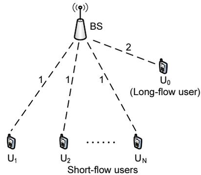
(a) A single-cell wireless downlink system with a long-flow user and multiple short-flow users.
