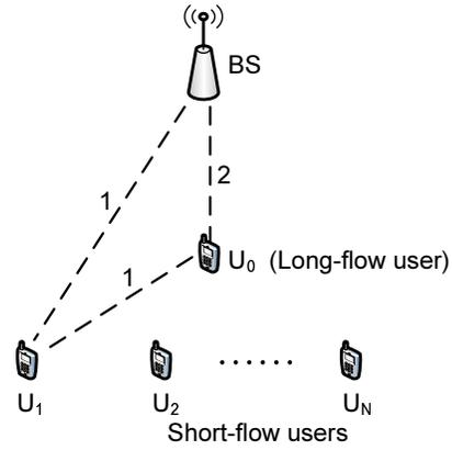
(a) A single-cell wireless downlink system with relay-assisted 2-hop communications. Note that the link between  $U_i$  and  $U_0$  and the link between  $U_i$  and the BS are similar to those for  $U_1$ , and are thus not displayed.
