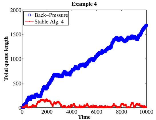
(b) Comparison of Q-BP and Stable algorithm 4 (i.e., the priority algorithm that gives a priority to the short flows), under the arrival rate vector of  $[p_l, p_s] = [0.5, 0.28]$ .
