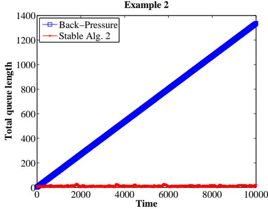
(b) Comparison of D-BP and Stable algorithm 2 (i.e., the Static Randomized scheduling algorithm as described in Example 2).
