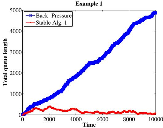
(b) Comparison of Q-BP and Stable algorithm 1 (i.e., the Static Randomized scheduling algorithm as described in Example 1), with  $B = 8$  and  $\epsilon = \frac{B-6}{12B(2B-3)}$ .
