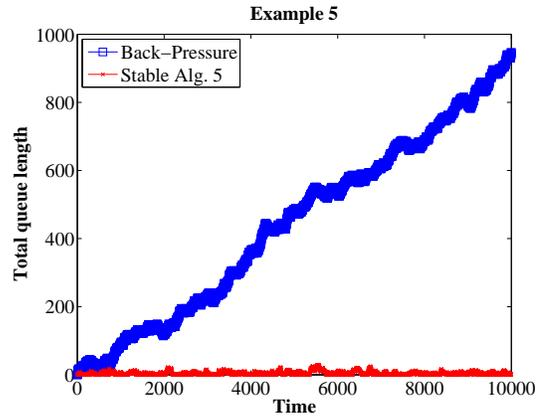
(b) Comparison of Q-BP and Stable algorithm 5 (i.e., the WSL algorithm with short flows using direct communications), under the arrival rate vector of  $[p_l, p_s] = [0.5, 0.2]$ .
